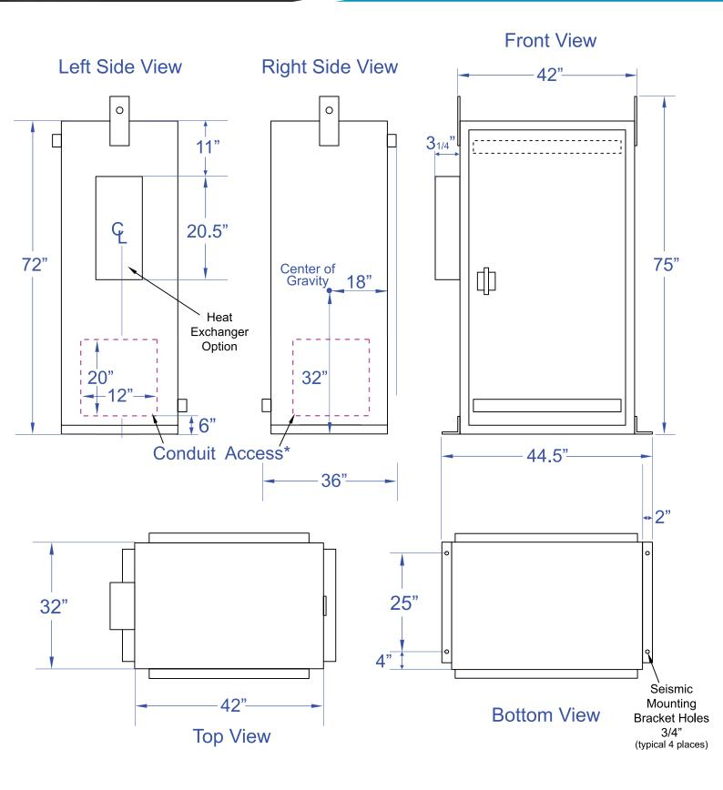
Per code requirements please leave 3" on each side of the cabinet including the back, and a 3 foot clearance in front.
