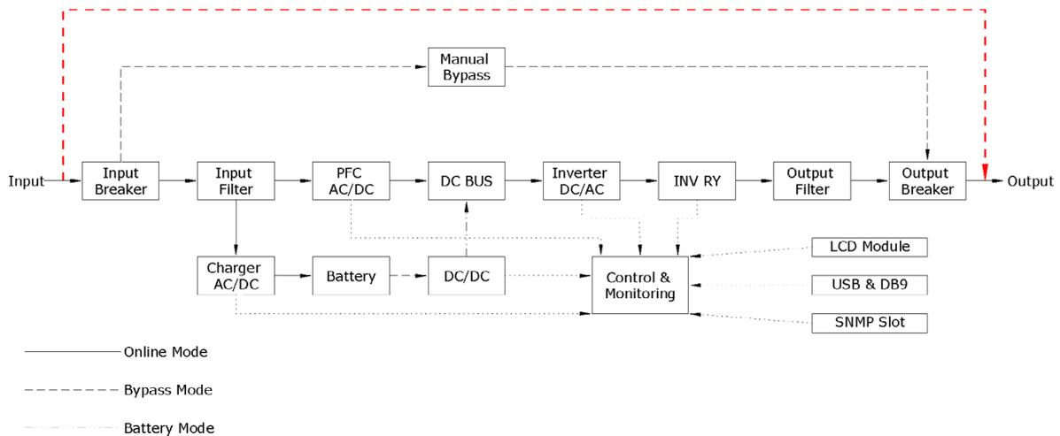
Figure 5 Single Line Drawings –External Maintenance Bypass Operation
